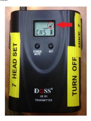
3. To change the channel on the transmitter please hold the "SET" button until the channel number is **FLASHING**. You must select the new channel while the number is flashing, it will only flash for **7 SECONDS**.
