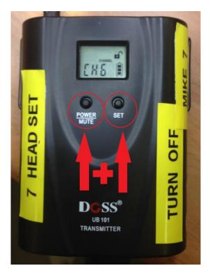
6. To **LOCK** the channel number in push the "POWER" and "SET" buttons **TOGETHER AGAIN.**This should now show the "PADLOCK" **LOCKED**. Now the channel number cannot be changed until you unlock the "PADLOCK" or reset the unit.
