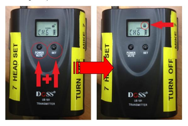
P.S. If you accidentally **LOCK** the wrong channel simply push the "POWER" and "SET" buttons **TOGETHER** to unlock the "PADLOCK". Now you can hold "SET" to change the channel again.
