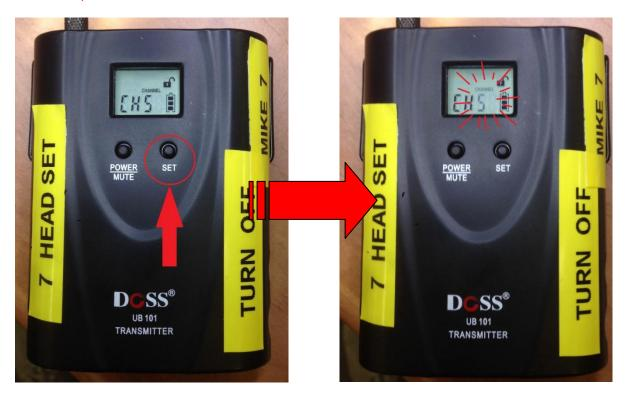
4. While the channel number is flashing keep pushing the "SET" button until you reach your desired channel. (Channel 6 is shown as an example).
