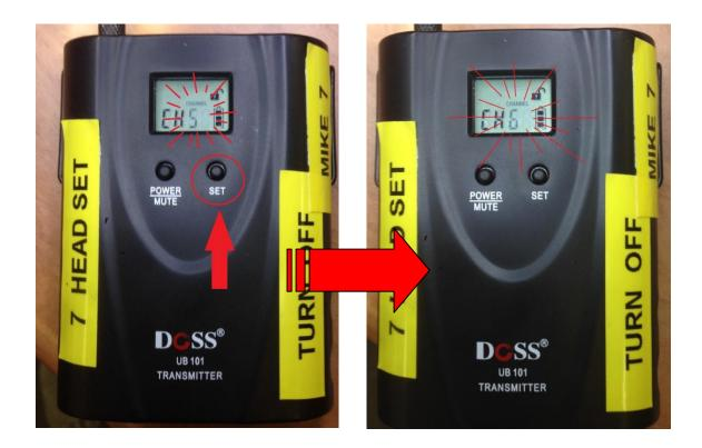
5. Once your desired channel number is on the screen push the "POWER" and "SET" buttons **TOGETHER** to set the channel number. The number will now **STOP** flashing.
