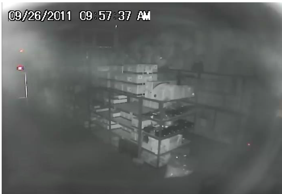
Demonstration of camera been too close to the edge of the camera dome cover
